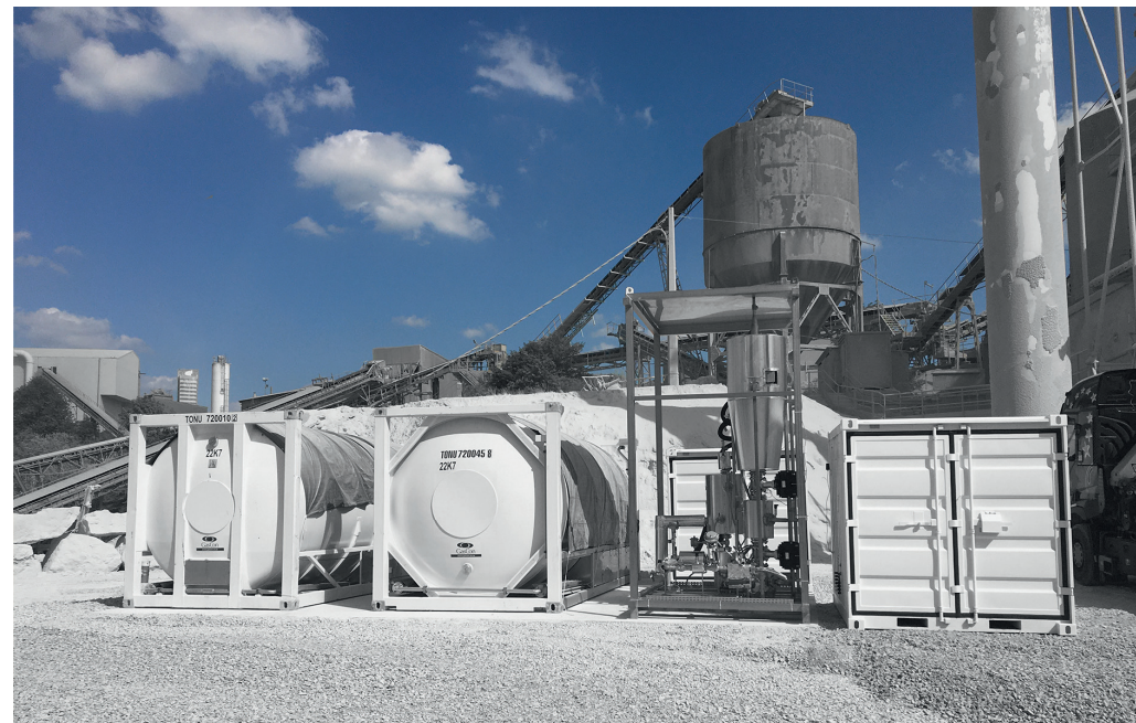
Lime factory located in Bocahut (Nord). The CO 2 capture system is shown in the centre of the picture. Two CO 2 storage tanks are visible to the left.
